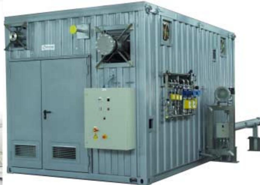
Natural gas purification and steam reforming for media supply for fuel element cell
